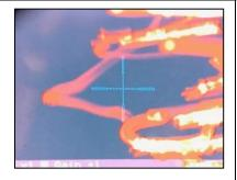
turned on! Doing so will permanently damage the sensor with random light glare (similar to pictured here). Such damage is not covered by the warranty and will void any warranty claims. Always have the protective cover on the scope when transporting it during daylight, particularly during sunny days! Always transport your scope during sunny day pointed downwards.
